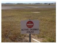
m) Aircraft Give way Markers are generally found at entry to the movement area to indicate that drivers must give way to aircraft.
